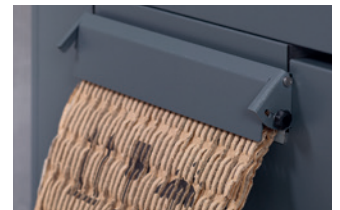
Creation of compressed packaging material with a closed compression flap (two layers of cardboard, HSM ProfiPack P425).
